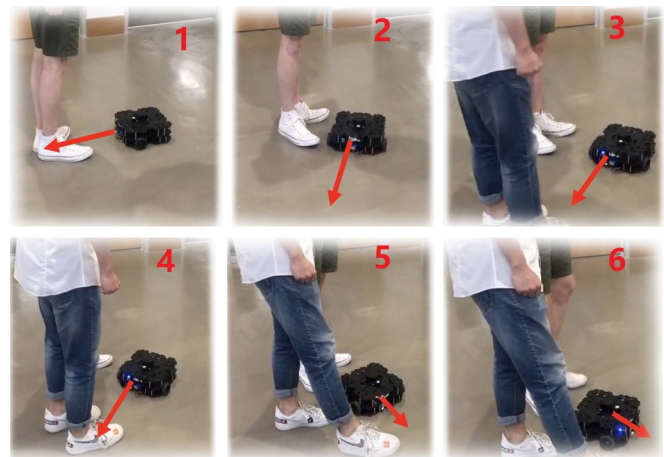
Fig. 8: A real-world deployment. We deploy our collision avoidance policy on turtlebot3. The red arrows represent the moving directions of the robot. The result shows that when two pedestrians try to maliciously block the robot, our trained collision avoidance policy still find a collision-free path for the robot.
