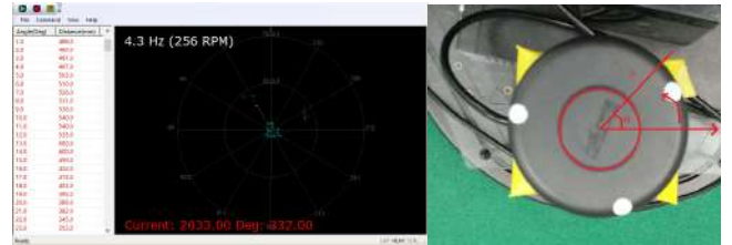
Fig.3. the internal polar coordinate space of the LIDAR
