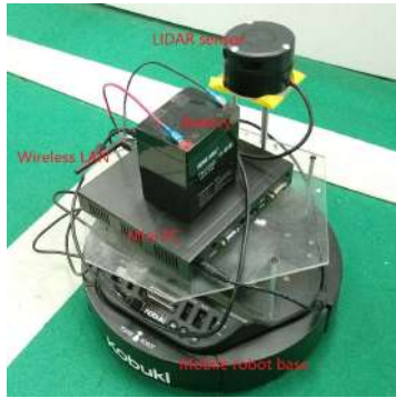
Fig.1. the robot platform and the LIDAR sensor
